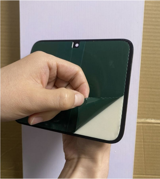
Image 1.1 Backplate adhesive. Peel the protective film
