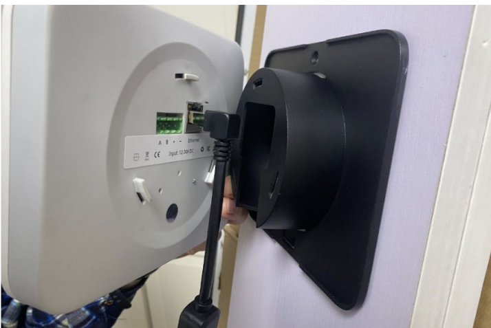
Image 1.8 Attach the sensor to the backplate (optional ethernet adapter shown)
